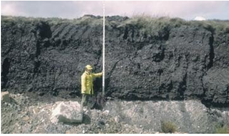
Peat overlying boulder clay, Plenmeller Opencast Coal Site © BGS, NERC.
