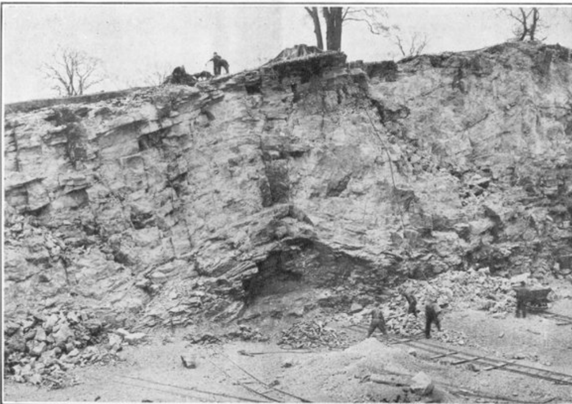
Plate 3B Same quarry, nearer view of face showing arching of strata, bedding and jointing.
