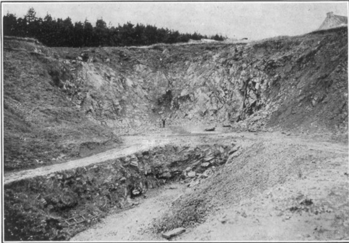
Plate 7A Drummuir Quarry, Banffshire. General view of quarry, showing method of working in two benches and dip of beds of limestone.
