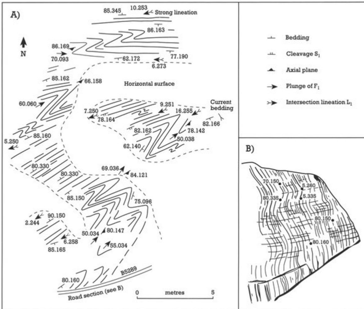
(Figure 3.4) Skiddaw Group exposures, near Buttermere. (A) is a horizontal surface. (B) Vertical roadside section in (A) looking towards 060^\circ . Three fold phases are represented in these exposures. The steep plunge of the folds represents the dip of a limb fold, initiated during F_0 . The D_1 phase is represented by the tight ENE–WSW folds and related cleavage, and D_2 by open recumbent folds and crenulation cleavage which can only be viewed on vertical surfaces, where the other two phases cannot be seen (after Moseley, 1981, and notes by D. Aldiss B.Sc. thesis, Birmingham University, 1974).
