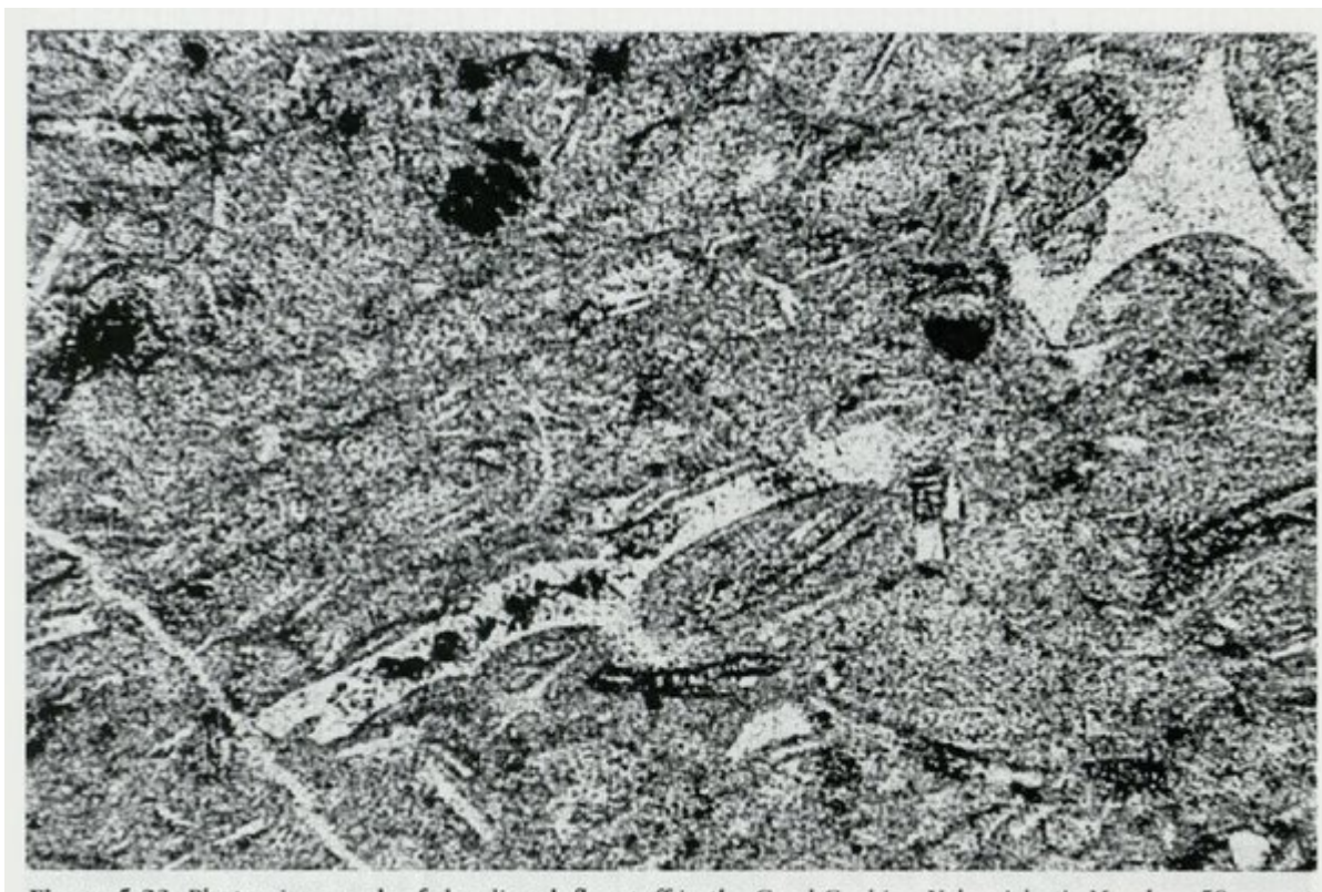
(Figure 5.23) Photomicrograph of shardic ash-flow tuff in the Coed Cochion Volcaniclastic Member, 50 m east of the disused quarry at [SN 3338 1463] (from Cope and Bevins, 1993).
