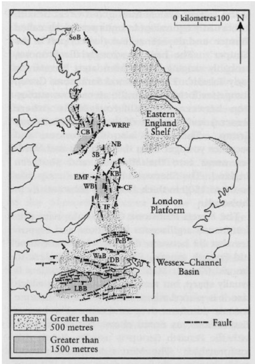
(Figure 1.5) The principal Permo-Triassic sedimentary basins and syndepositional normal faults in England. Intensity of stippling indicates sediment thicknesses. Abbreviations: CB, Cheshire Basin; CF, Clopton Fault system; DB, Dorset Basin; EMF, East Malvern Fault; IF, Inkberrow Fault; KB, Knowle Basin; LBB, Lyme Bay Basin; NB, Needwood Basin; PeB, Pewsey Basin; SB, Stafford Basin; SoB, Solway Basin; WaB, Wardour Basin; WB, Worcester Basin; WRRF, Wem-Red Rock Fault system.
