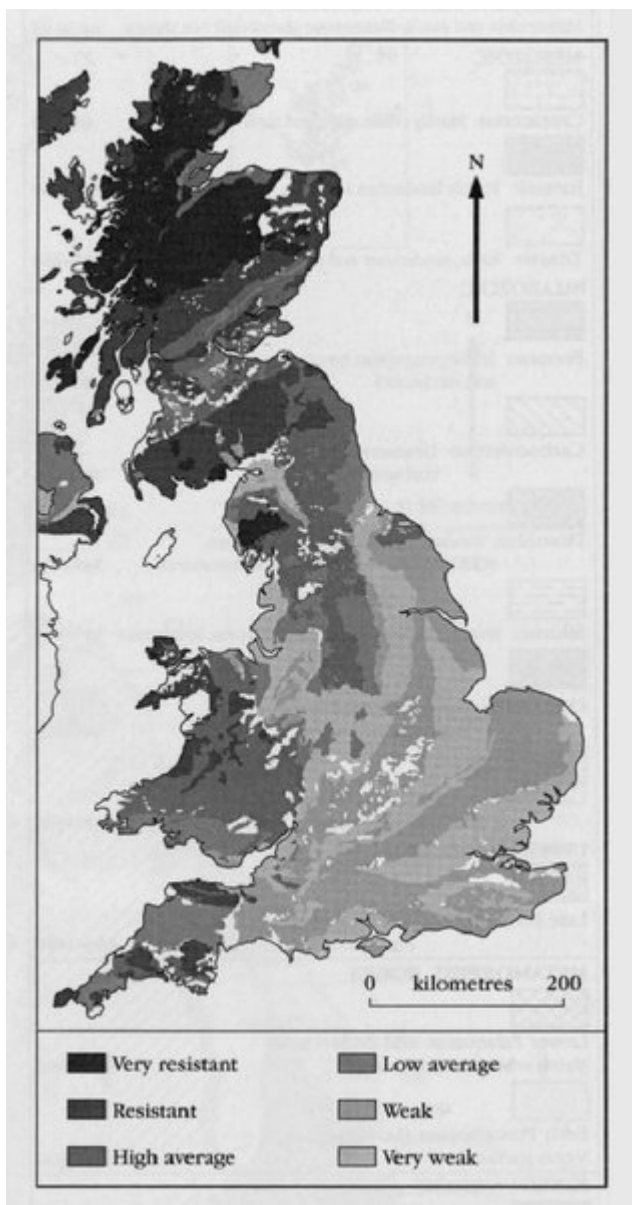
(Figure 1.3) Relative rock resistance for 71 different outcrops (divided by lithology and age) was established through computer analysis of data on altitude, dissection, and geology for a grid of kilometre squares covering Great Britain and the surrounding continental shelf. Six consistent classes were established using up to 19 variables in various combinations. White areas are unclassified. (From Clayton and Shamoon, 1998, fig. 1).
