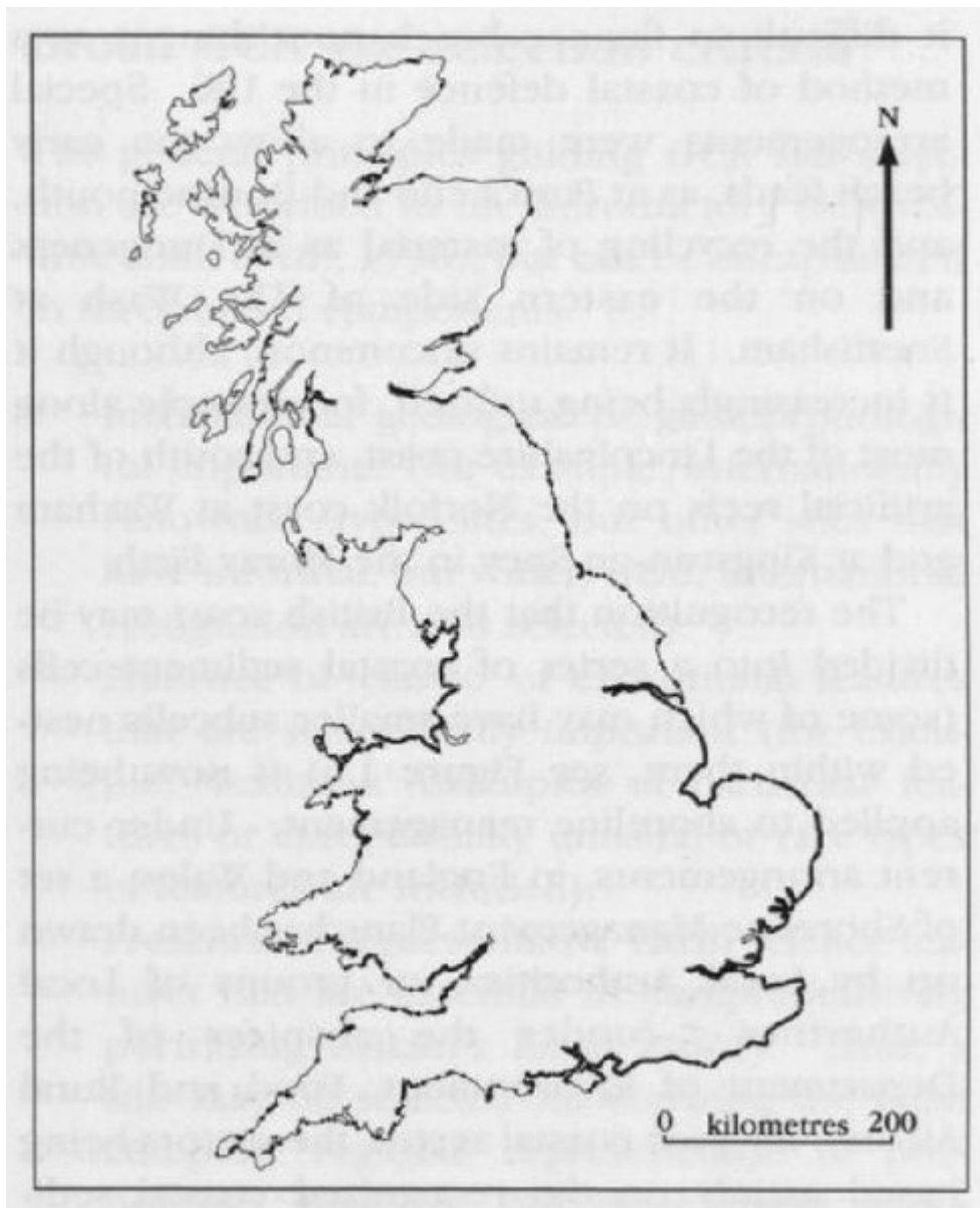
(Figure 1.9) Coastal engineering structures in Britain ('coastal protection' and 'sea defences'), shown as coastline with heavier line weight. Note the concentration on south-eastern England, Bristol channel, and north Wales and north-west England. (Data from Halcrow Group Ltd for England and Wales, published with permission from Department for Environment, Food and Rural Affairs; Scottish data after Ramsey and Brampton, 2000a-f.)
