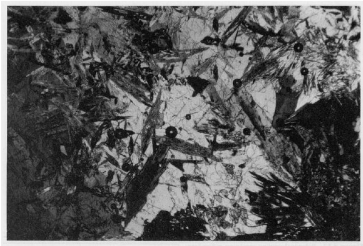
(Figure 4.14) Photomicrograph of mineral relationships in late amphibole-rich hydrothermal veins, near Clodgy Point, Penwith Peninsula (cross polars). (Photo: P.A. Floyd.)
