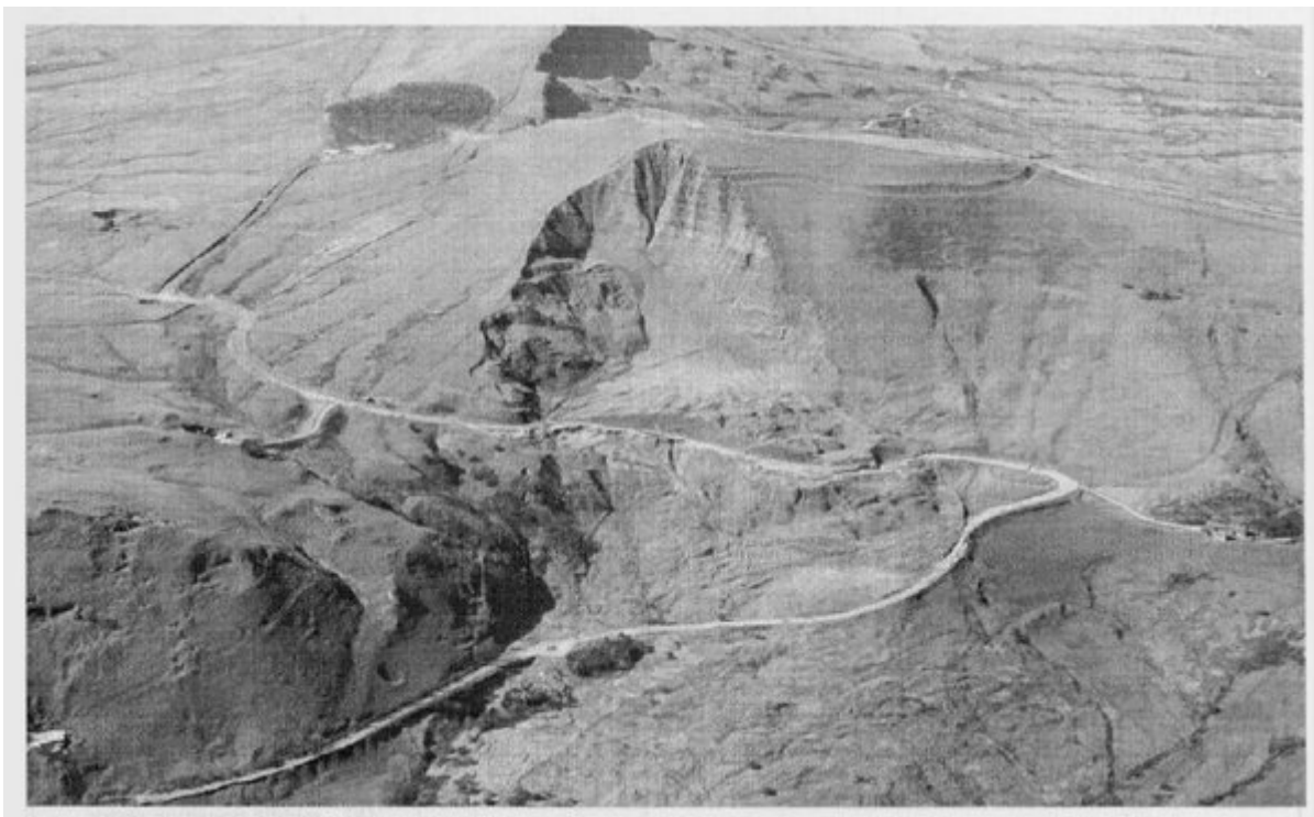
(Figure 5.27) Oblique aerial photograph of the Mam Tor area, showing the old road which was closed in 1979 owing to repeated slippage. The scar of the landslip is clearly visible, as well as a slumped mass. (Photo: © National Trust/High Peak.)
