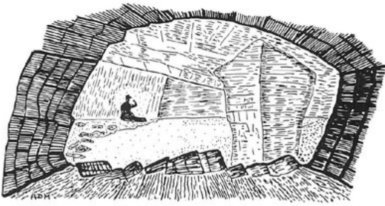
(Figure 21) The Old Town Hall, Bo'ness, and stoop and room workings in the Western Main Coal 15 m below the Old Town Hall, after Cadell 1925.
