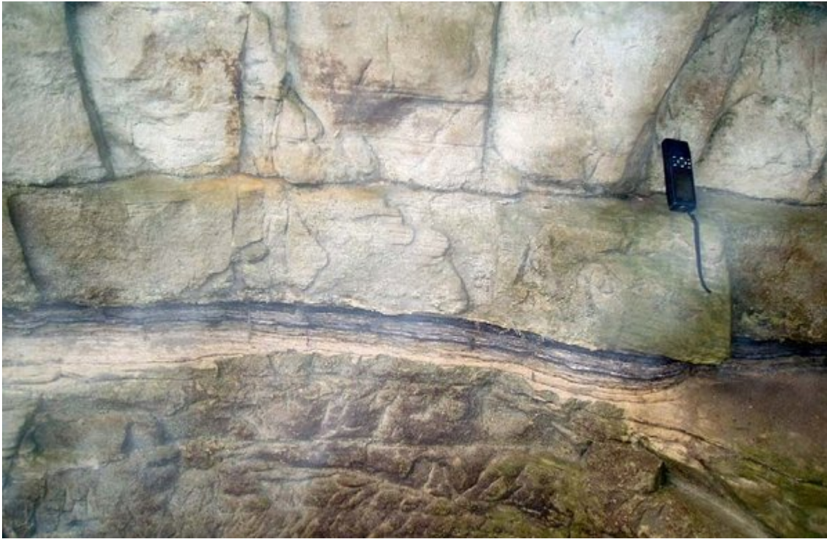
(Figure 40) Obelisk Quarry, Hopetoun [NT 0942 7859] (WLGS 13). Close-up of (Figure 39). Fine grained sandstone with interbeds of very fine grained sandstone and laminated carbonaceous siltstone ("tiger-stripe").
