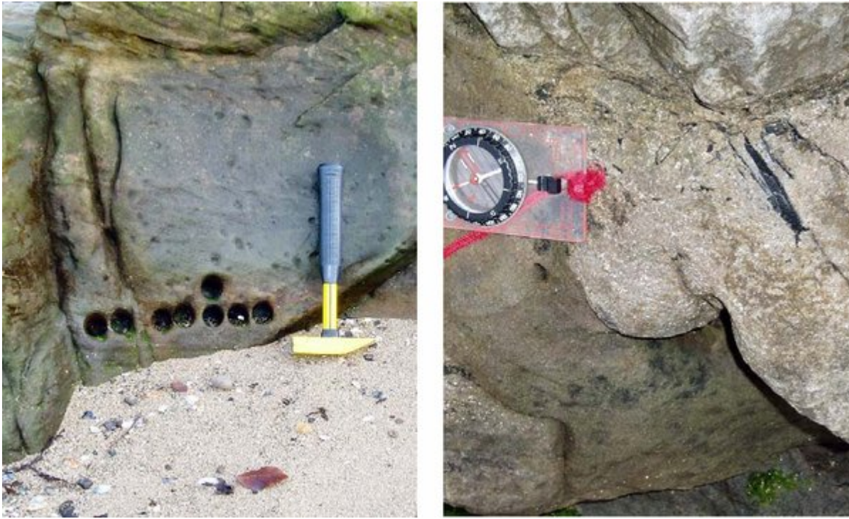
(Figure 50) A: Damage to sandstone caused by core-cutting. B: Close-up of (Figure 49) — carbonaceous lags (plant debris) in sandstone. Society Point, Binny Sandstone, Hopetoun Member, West Lothian Oil Shale Formation [NT 1009 7902] (WLGS 15).
