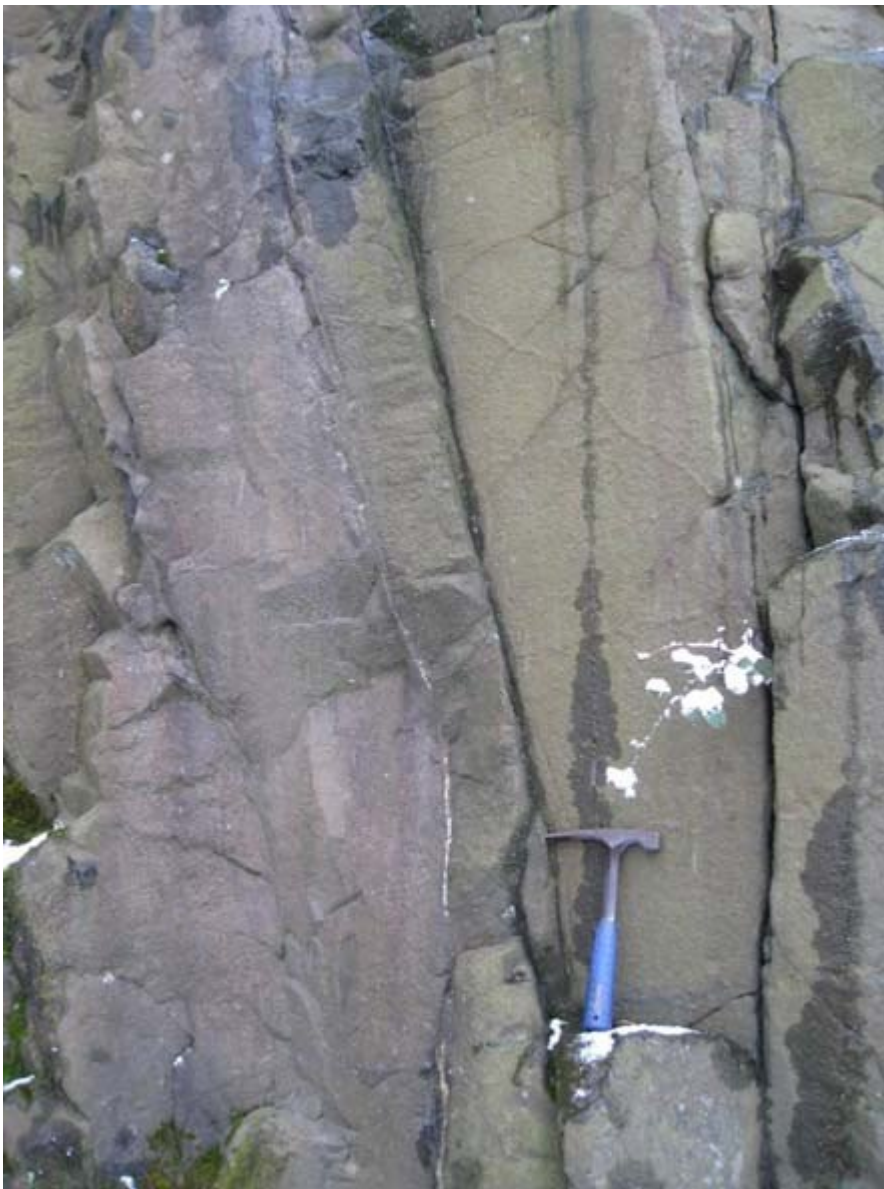
(Photo 3) A network of quartz and calcite veins within the quartz-microgabbro. Looking N.
