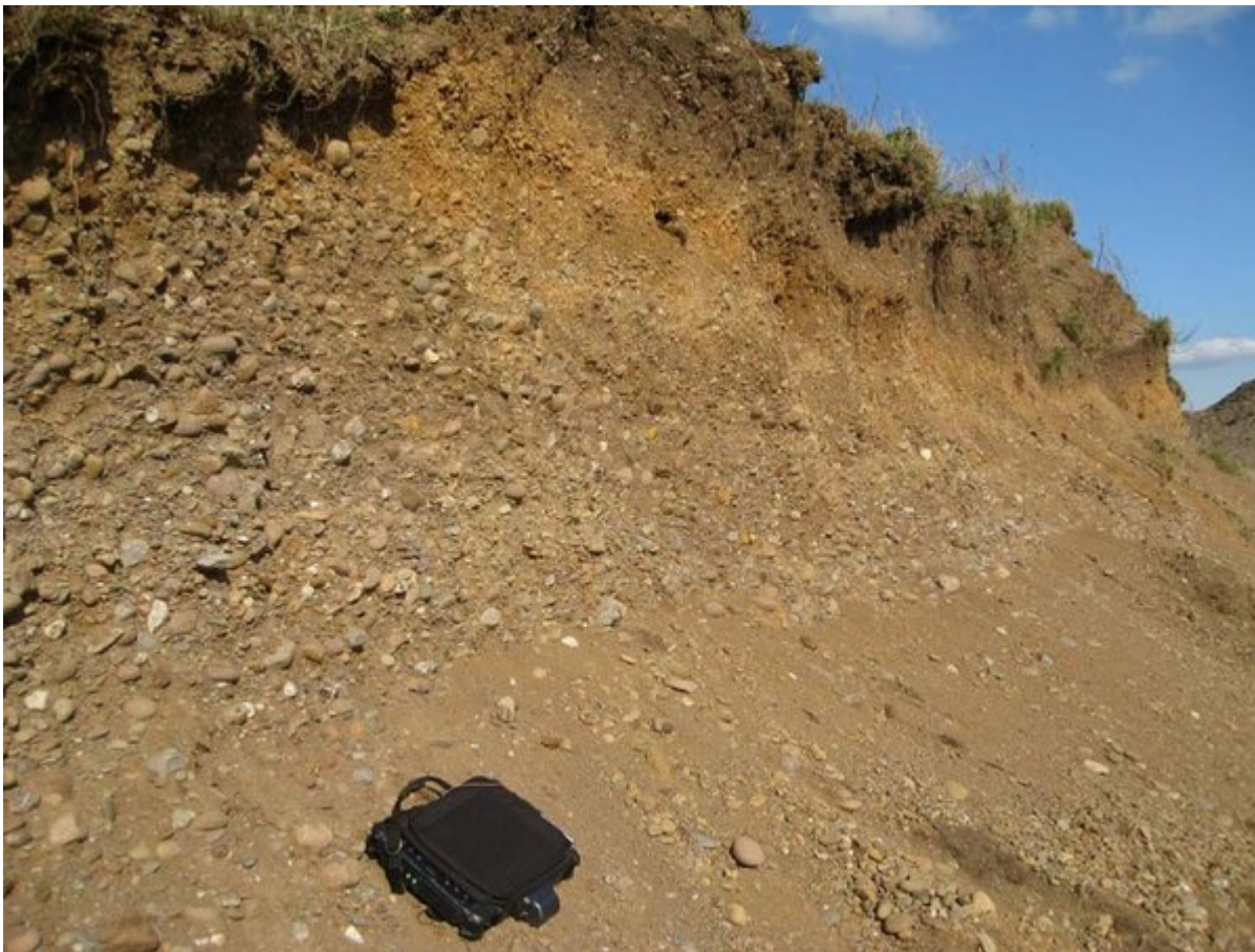
(Photo 181) Exposures in the upper gravel unit, seen along the north eastern edge of an area which is partly infilled. The section displays up to 4 m of sandy gravel. Looking ENE.
