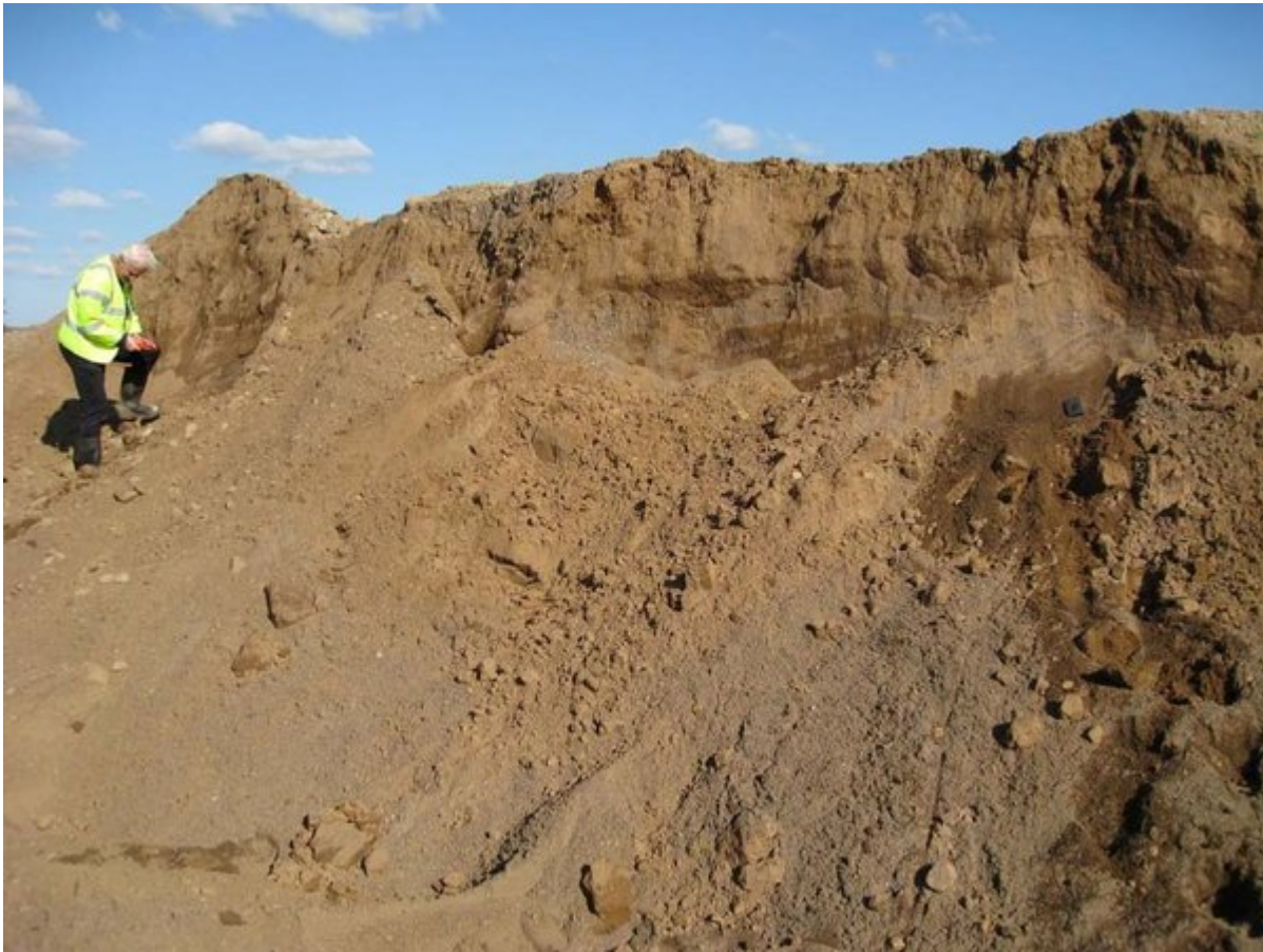
(Photo 183) Exposure in the lower sand unit at the southern edge of the active quarry (the upper gravel unit has been removed). On this visit approximately 1m of bedded medium- to coarse-grained sand with fine gravel was exposed. Looking east.
