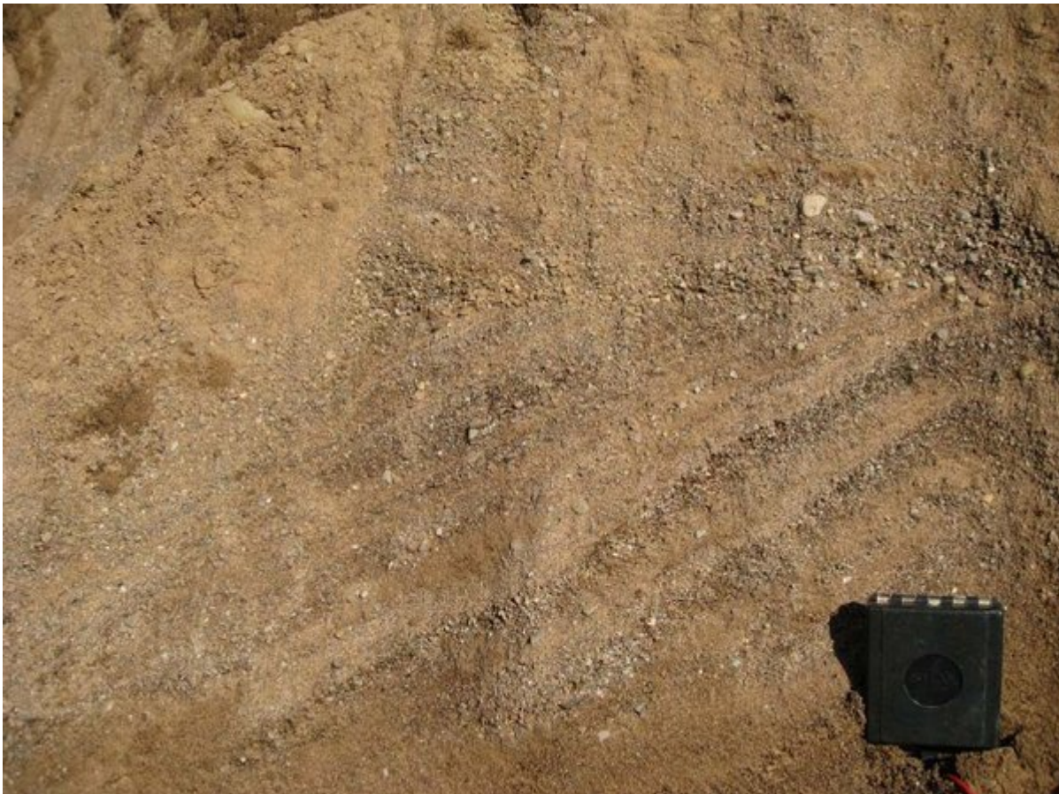
(Photo 183) Exposure in the lower sand unit at the southern edge of the active quarry (the upper gravel unit has been removed). On this visit approximately 1m of bedded medium- to coarse-grained sand with fine gravel was exposed. Looking east.
