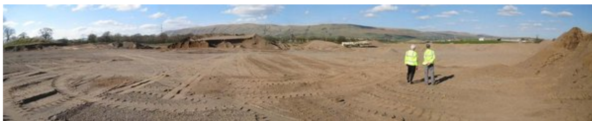
(Photo 179) Panorama across the active area of the quarry, with the Campsie Fells and Kilsyth Hills in the distance. The quarry is exploiting the glaciofluvial sand and gravels belonging to the Broomhouse Formation. Across the area the deposit is only a few metres thick and is generally composed of gravels overlying a unit of sand.
