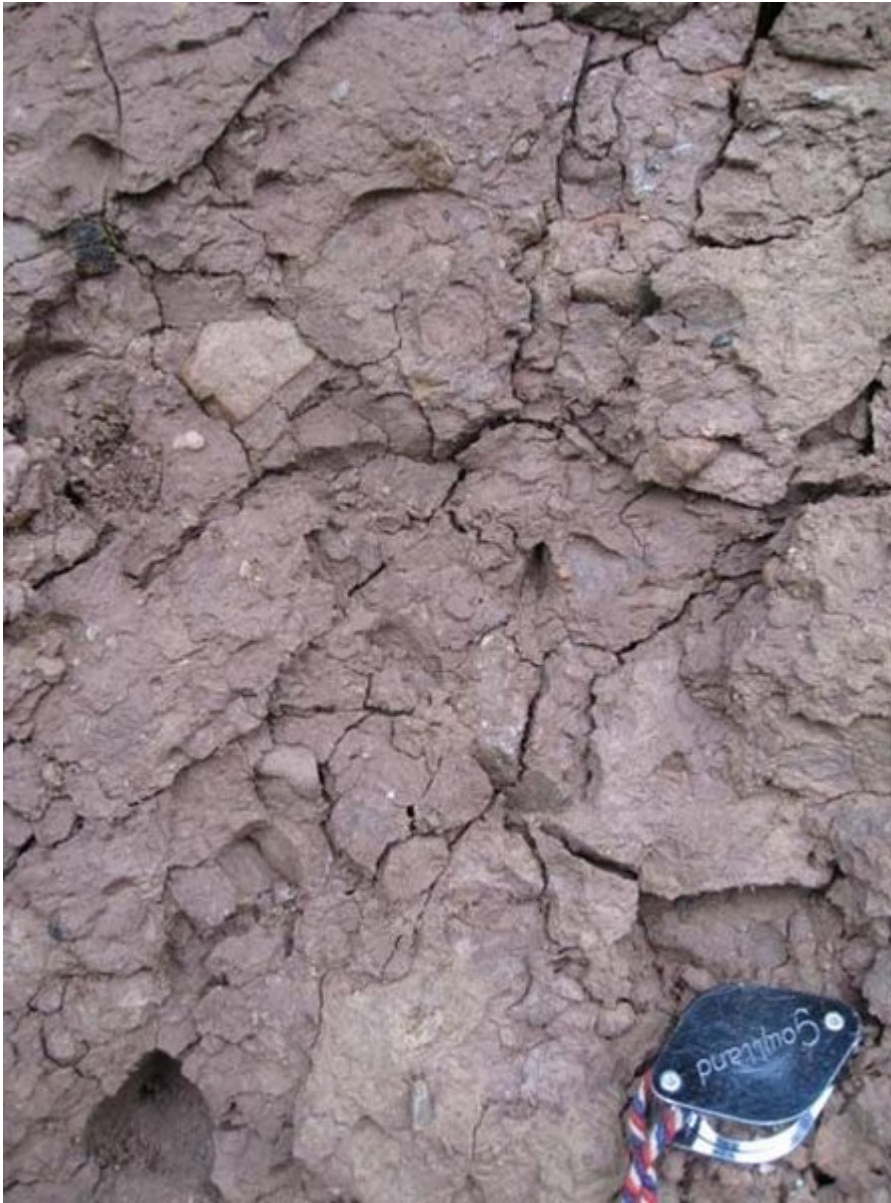
(Photo 201) Close-up of the Wilderness Till Formation, showing fractures in the over- consolidated glacial till.
