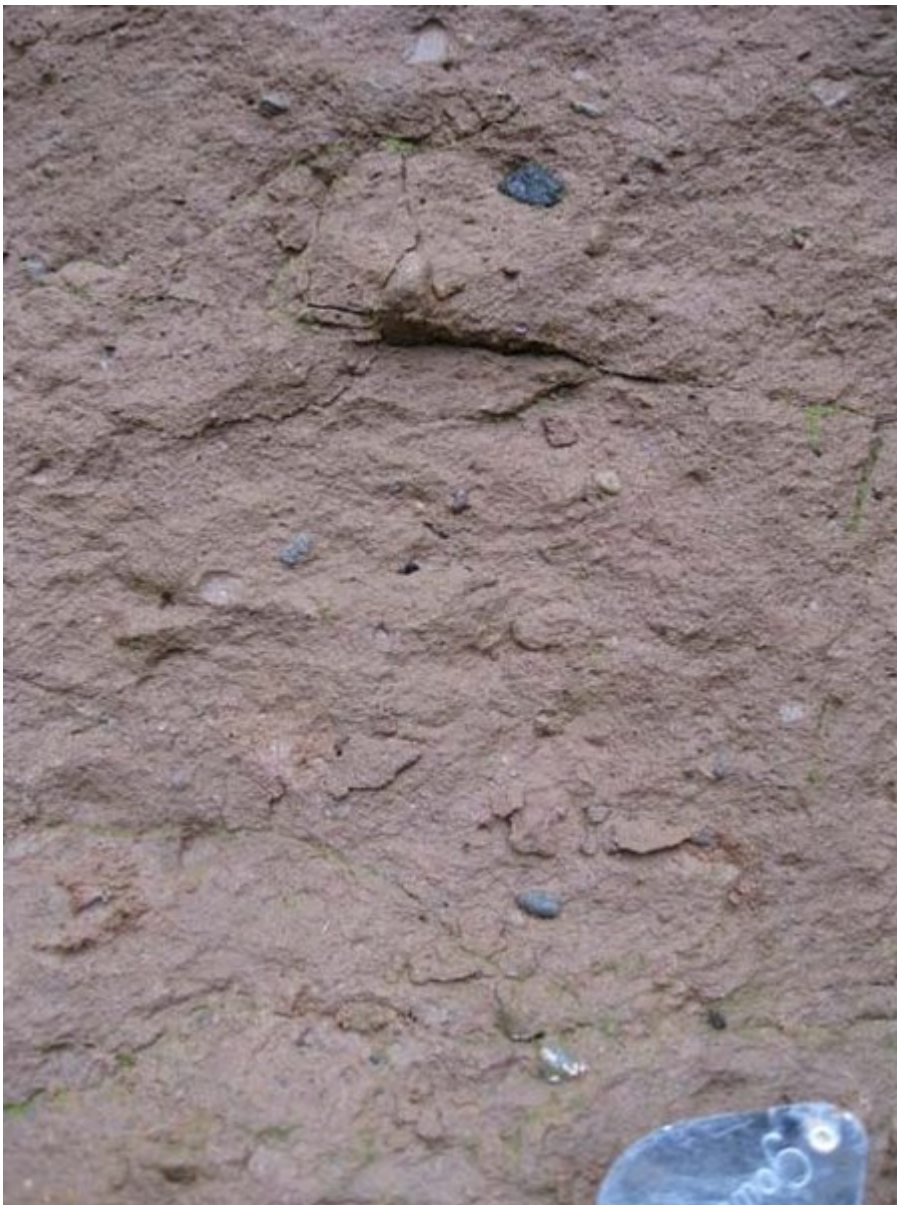
(Photo 202) Close-up of the Wilderness Till Formation, showing the nature of the matrix of the glacial till; sandy with scattered gravel.
