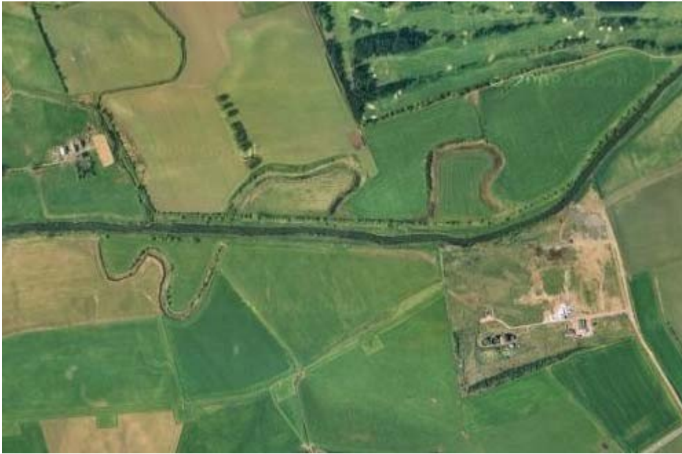
(Photo 220) Aerial view of three remnant meanders, abandoned when the River Kelvin channel was artificially straightened.
