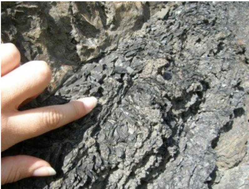
(Spireslack_2 P4) Internal fractures display heavily polished surfaces, evidence of the rocks on either side moving past each other (see right image). © BGS, NERC.
