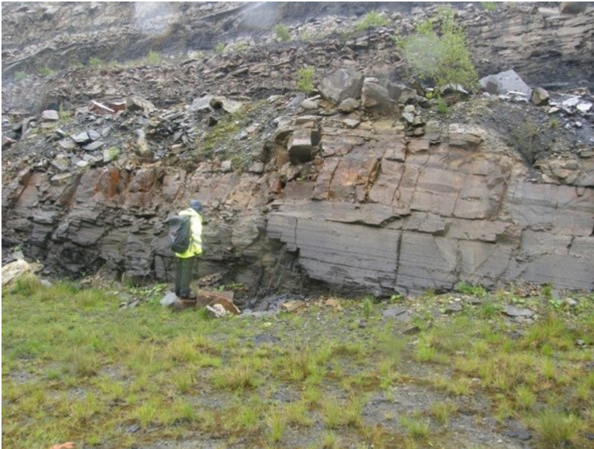
(Spireslack_12 P1) Section of Limestone Coal Formation, showing a 5 metre coarsening upward sequence through mudstones to sandstones. © BGS, NERC.
