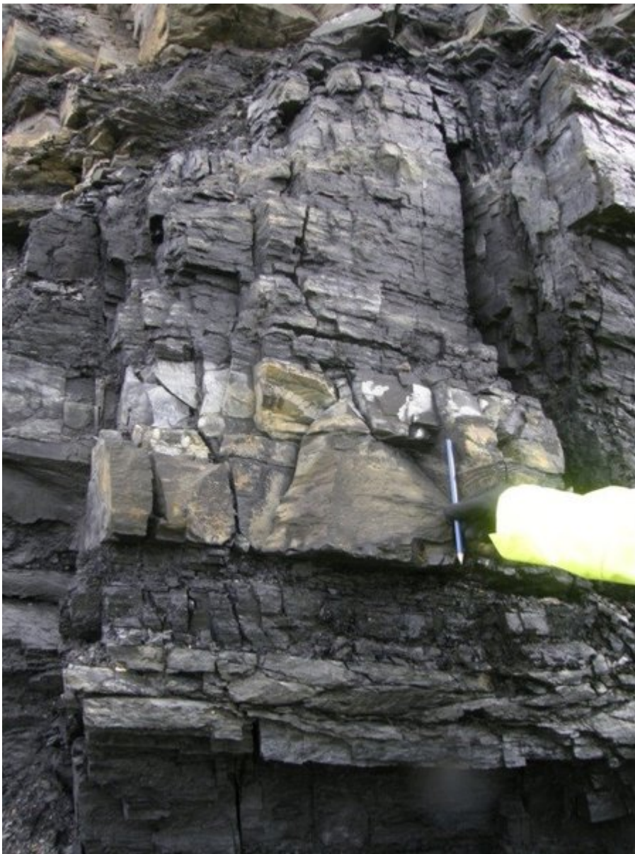
(Spireslack_13 P1) 20 cm thick band of cannel coal set within the Muirkirk Nine Foot Coal seam. © BGS, NERC.
