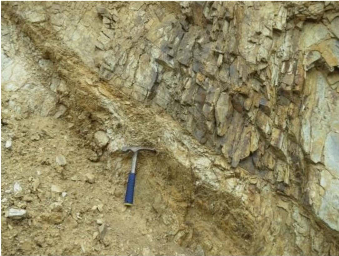
(ELC_1_P5) A 10cm wide fault zone is exposed at the north end of the east wall, composed chiefly of brecciated clasts of the surrounding siltstone. Photo taken looking west. © BGS, NERC.
