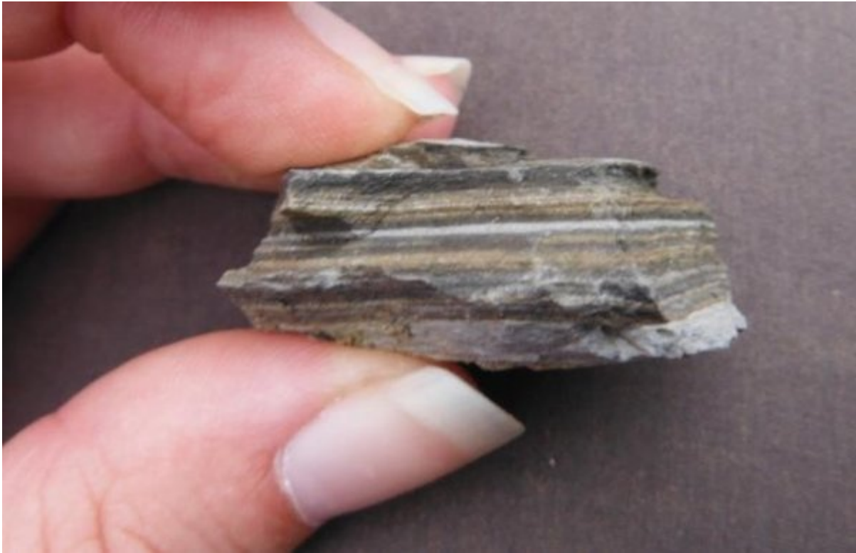
(ELC_1_P1) Steeply dipping, thinly bedded siltstones, mudstones and shales exposed in the east wall of the quarry at Gala Law. The thicker units are grey-brown siltstone, with thinner black shale and pale grey micaceous mudstone between. These sequences represent low-density submarine turbidity current deposits, resulting from low-concentration flows transporting mainly silt- and clay-sized material. These fine-grained sediments would have been deposited by
