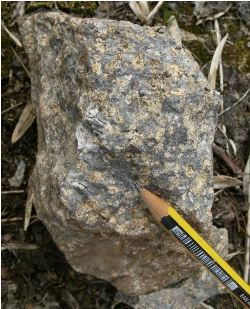
(ELC_12_P8) Close up of the porphyritic trachyte which was extracted from the quarry and used to construct many of Haddington's stone buildings. © BGS, NERC.
