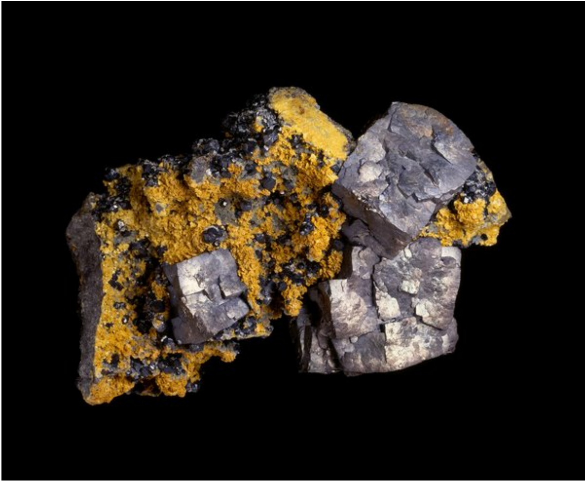
(Photo 53-1) Lead and zinc ores (galena and sphalerite) from Nenthead mines.
