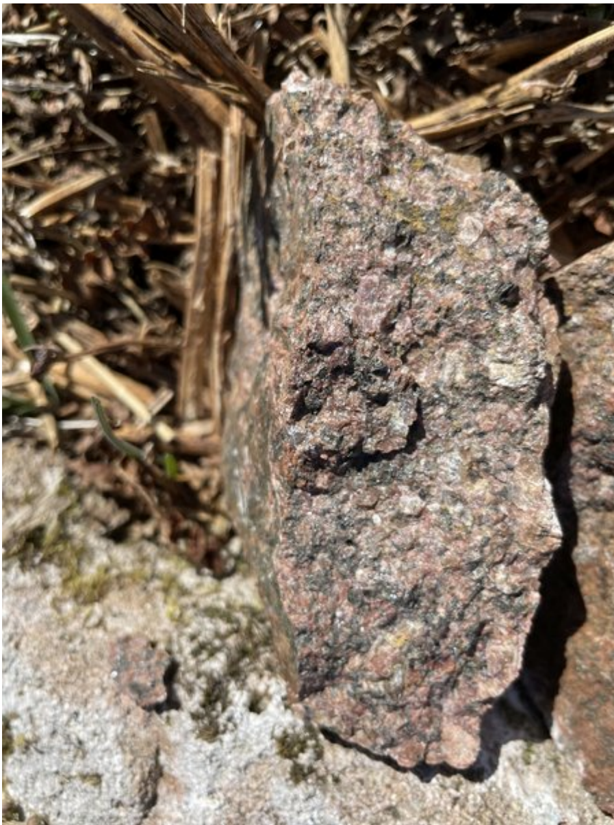
(Photo 18-1) Cheviot Granite. Large interlocking crystals of quartz, feldspar and biotite.
