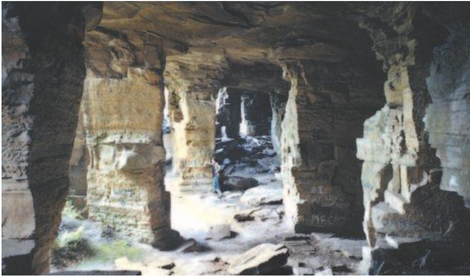
(Photo 19) Hown's Quarry, Consett. Underground quarries in the sandstone between the Marshall Green and Victoria coals. BGS, ©NERC, 2004.
