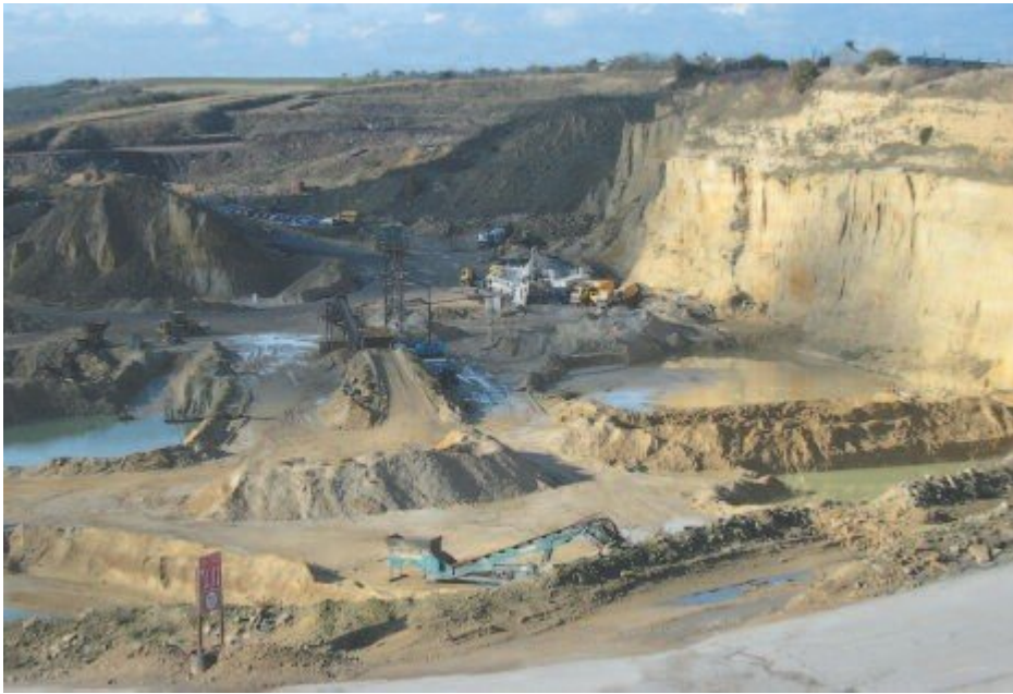
(Photo 22) Crime Rigg Quarry, Sherburn Hill. Thick Yellow Sands beneath Raisby Formation and Marl Slate. DJD Lawrence, BGS, ©NERC, 2004.
