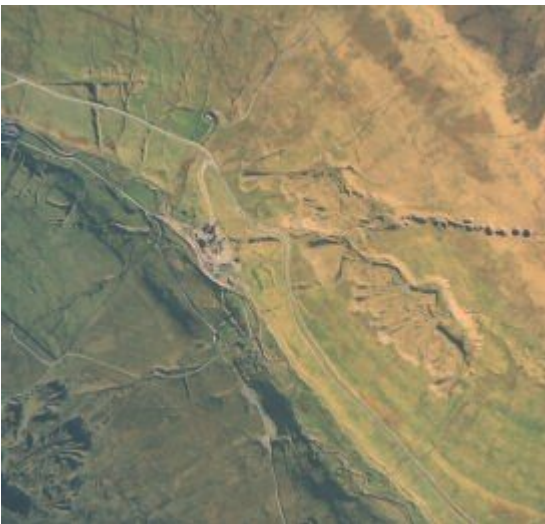
(Photo 48) Aerial view of Groverake Mine, Rookhope. The course of Groverake vein is marked at the surface by a line of large crown holes. Infoterra.
