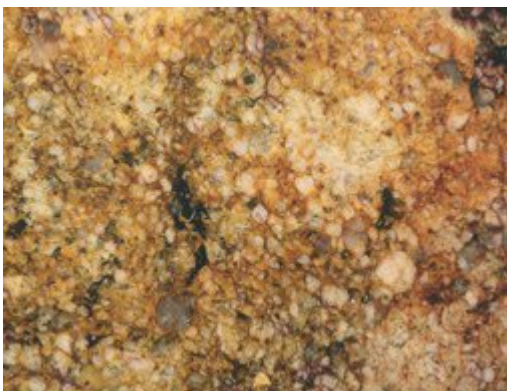
Polished slab of the breccia matrix, showing abundant white quartz and feldspar crystals.
