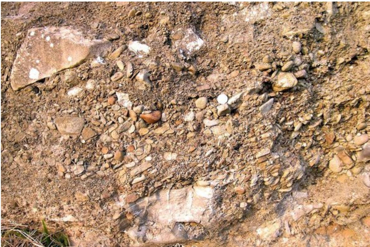
(Figure 74) Exposure E - detail of cemented coarse glacial sand and gravel, showing imbricated pebbles. [SK 51713 99601].
