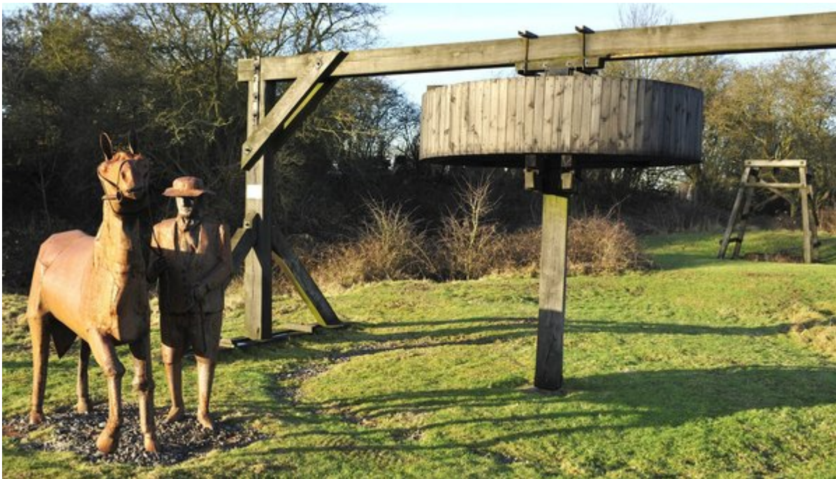
(Figure 96) Model horse and winding gear for extracting coal from a bellpit. In the background is a former bellpit with winding gear.
