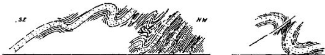
FIGS. 205, 206.—NORTH-WESTWARD FACING ISOCLINES IN ARENIG BEDS BELOW THE BODAFON THRUST-PLANE.
