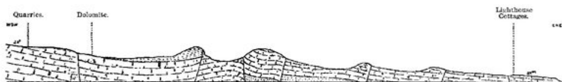
FIG. 301.—SECTION ALONG THE COAST FROM THE PENMON QUARRIES TO THE EAST POINT OF ANGLESEY. Scale—16 inches = one mile. d_1, d_2, d_3 = D_1, D_2, D_3 sub-zones of Carboniferous Limestone.
