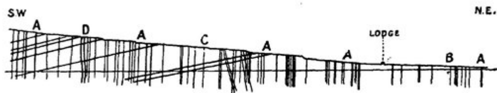
FIG. 8.—Section along Allt Dearg Mòr, near Sligachan: scale, 1\frac{1}{2} inch to a mile. The general direction is N.E.-S.W., but the line is made to follow the principal bends of the stream. A number of dykes and a few thin sills are shown, the latter indicating the general dip of the lava-group.
