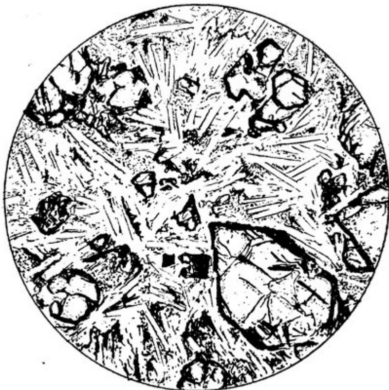
FIG. 7.—[9359] \times 20 . Olivine-Basalt lava, in Allt Dearg Mòr, about 2 miles S.W. of Sligachan: showing pseudomorphs after olivine, composed of carbonates with a border of iron-oxide.
