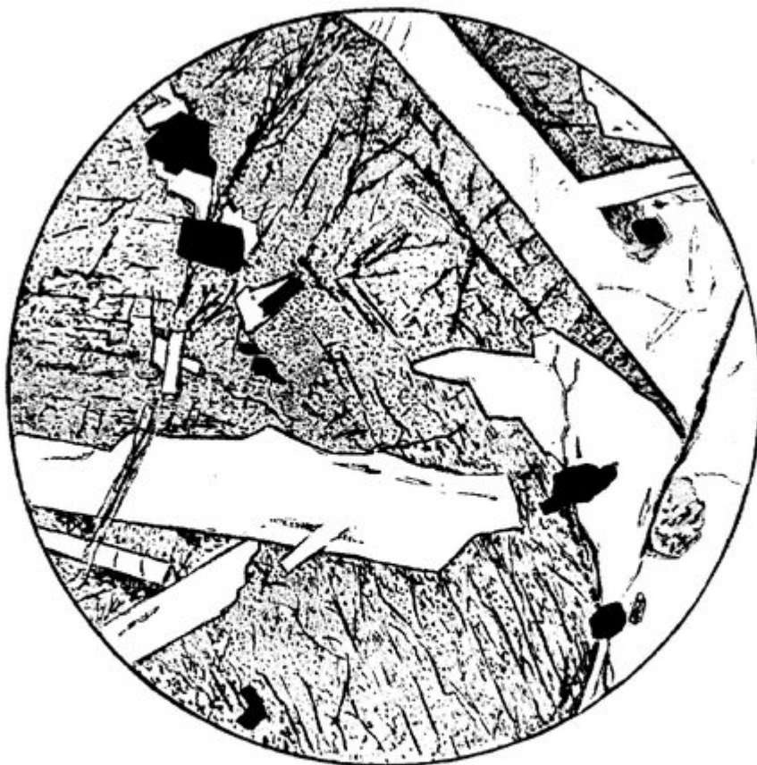
FIG. 68.—[5421] \times 30 . Diabase or coarse dolerite, dyke \frac{1}{2} mile E.S.E. of summit of Ben Aslak and 2 miles S.W. of Kylerhea. Typical ophitic structure. The feldspar crystals in this and numerous similar rocks show between crossed nicols a strong zonary banding, which does not disappear with the albite-lamellation, and is therefore due to the marginal portion being of different composition from the interior.
