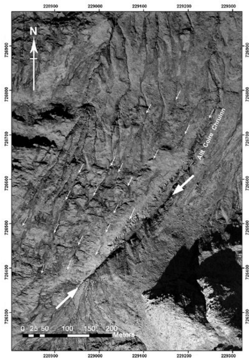
(Figure 3.58) Vertical aerial photograph of the northern flank of Ben Oss, showing the Ben Oss Fault (stream gully in centre with large arrows at each end) and fractures orientated at 20° anticlockwise to the fault on its north-west side (indicated by small arrows). See text for explanation. (Aerial Photograph © Getmapping.)
