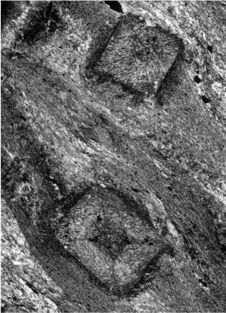
(Figure 6.24) Chiastolite (=andalusite) porphyroblasts pseudomorphed by fan-like sheaves of kyanite in a sample of pelite from the Mortlach Graphitic Schist Formation close to Auchindoun Castle. The original 'crosses' formed by graphite inclusions in the chiastolite are still clearly visible. (from Beddoe-Stephens, 1990, figure 2a). (Photo: BGS No. P 254543, reproduced with the permission of the Director, British Geological Survey, © NERC.)
