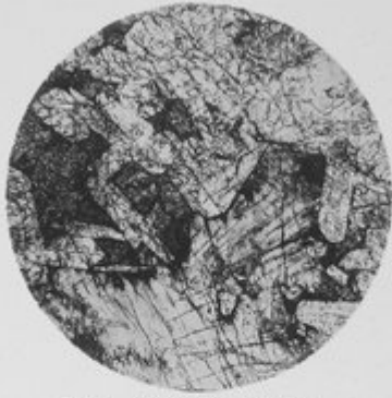
Fig. 1. Ophitic Dolerite. \times 14 .
