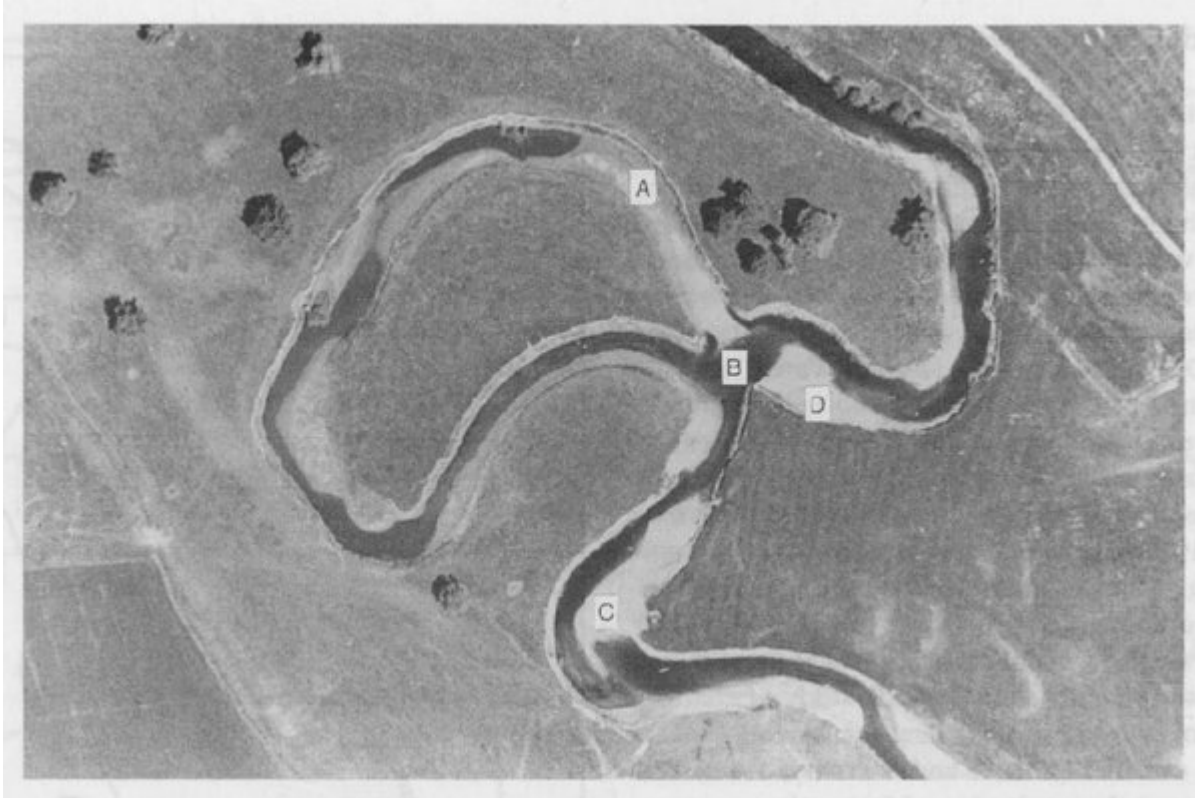
(Figure 2.18) A recent meander cutoff on the Endrick Water (October 1983). The abandoned channel has been plugged by sediment at the downstream end (A). The neck of the former floodplain (B) is now a riffle between a point bar (C) and a concave bench (D). (Photo: Royal Commission on the Ancient and Historical Monuments of Scotland; print 048, 514 88; flown June 1988: Crown Copyright.)
