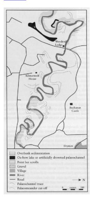
(Figure 2.17) Endrick Water: a geomorphological map of point bars, overbank sedimentation, point bar scrolls, oxbow lakes and palaeochannels. (Based on 1988 aerial photographs.)
