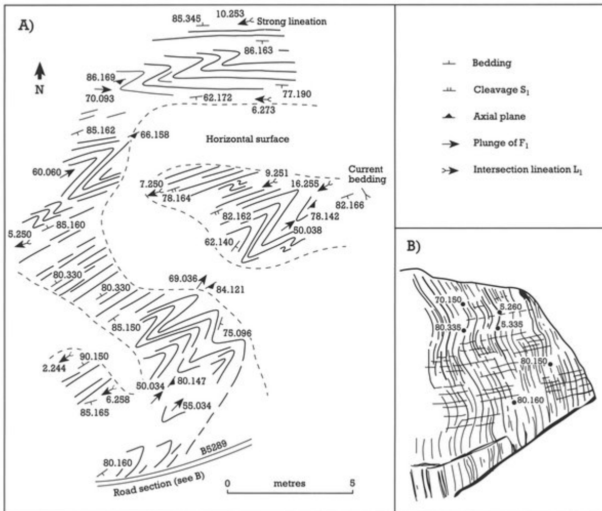
(Figure 3.4) Skiddaw Group exposures, near Buttermere. (A) is a horizontal surface. (B) Vertical roadside section in (A) looking towards 060°. Three fold phases are represented in these exposures. The steep plunge of the folds represents the dip of a limb fold, initiated during F_0 . The D_1 phase is represented by the tight ENE–WSW folds and related cleavage, and D_2 by open recumbent folds and crenulation cleavage which can only be viewed on vertical surfaces, where the other two phases cannot be seen (after Moseley, 1981, and notes by D. Aldiss B.Sc. thesis, Birmingham University, 1974).
